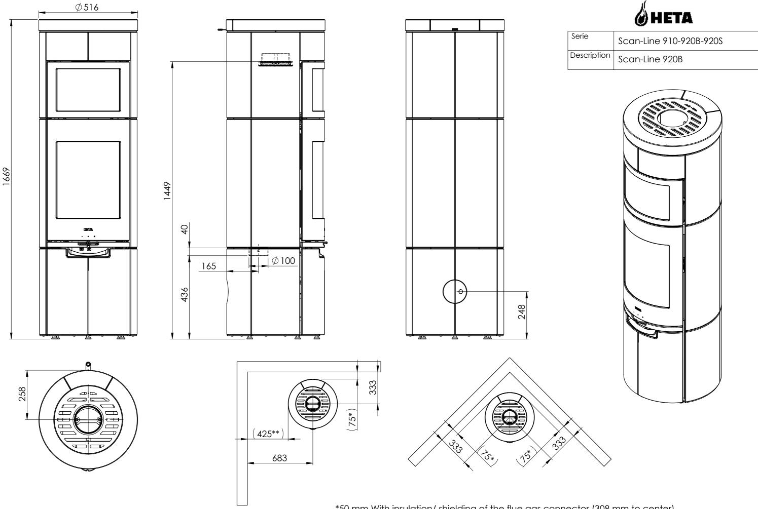
\*50 mm With insulation/ shielding of the flue gas connector (308 mm to center) \*\*400 mm With insulation/ shielding of the flue gas connector (658 mm to center)
